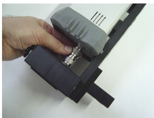
Fig. 10-12 Screwing the N-N Adapter for Antenna Matching
