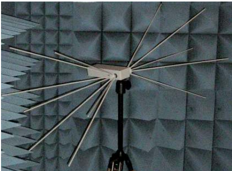
PMM BC-01 Biconical Antenna 30 - 200MHz
