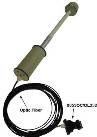
Fig. 2-2 OR-03 link with 8053-OC
