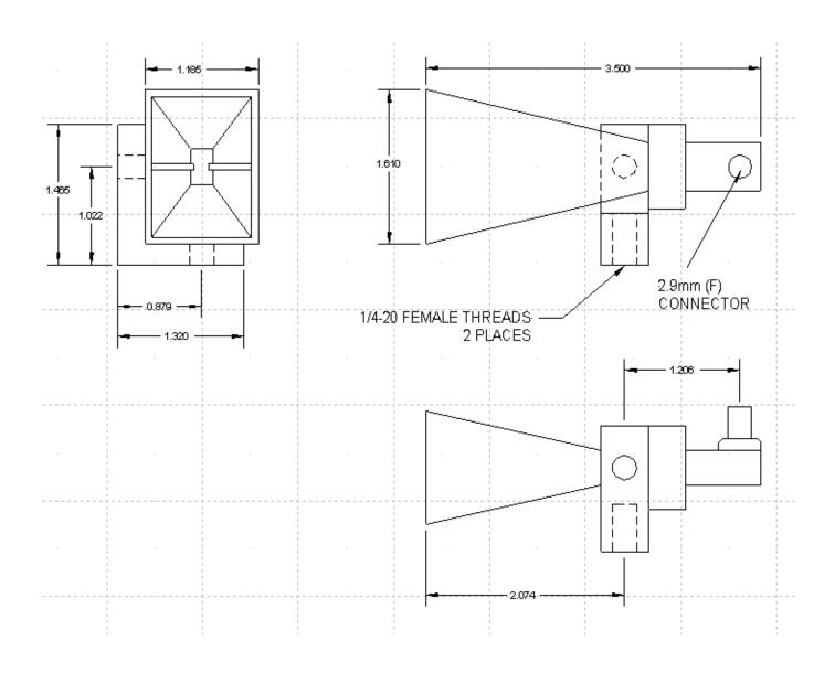
Physical Dimensions: Length: 3.5 in. (8.9 cm) Width:1.2 in. (3 cm) Height:1.6 in. (4.1 cm) Weight:0.2 lbs. (0.09 kg)
