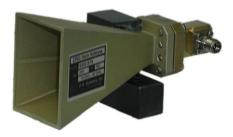
Frequency Range:18 GHz - 40 GHz Antenna Factor:40.3 to 41.1 Gain:15 to 21.2 dBi Maximum Continuous Power:10 Watts Max Radiated Field:150 V/M Impedance:50  $\Omega$ VSWR:1.2:1 (1.5:1 max) Connector:WRD-180C24 to 2.9mm female Mounting Base:1/4 - 20 Thread, female
