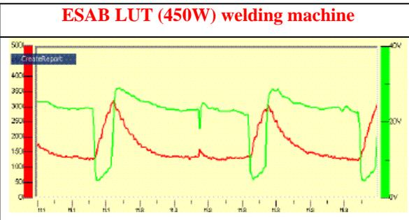
Figure 4: Voltage (green) and current (red) waveform
