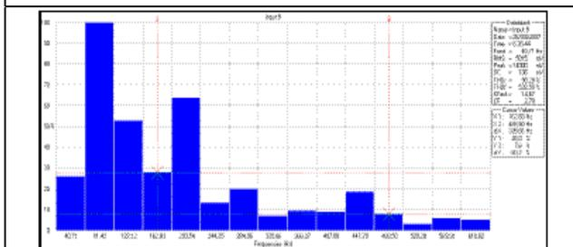
Figure 3: Harmonics with fundamental frequency of 81.42 Hz
