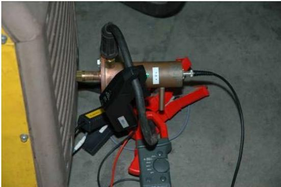
Welding machine with shunt and current clamps
