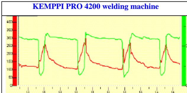
Figure 1: Voltage (green) and current (red) waveform
