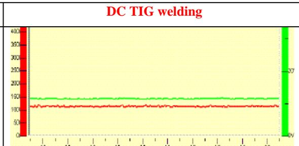
Figure 16: Voltage (green) and current (red) waveform
