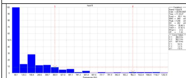
Figure 15: Harmonics with fundamental frequency of 60.1 Hz
