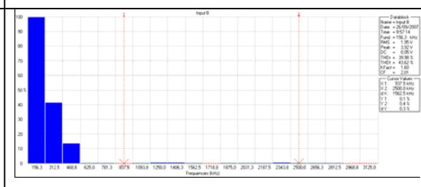
Figure 18: Harmonics with fundamental frequency of 156.3 Hz
