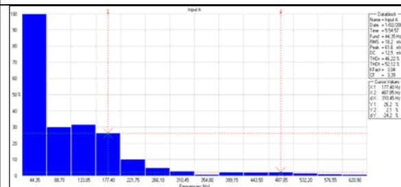
Figure 6: Harmonics with fundamental frequency of 44.35 Hz
