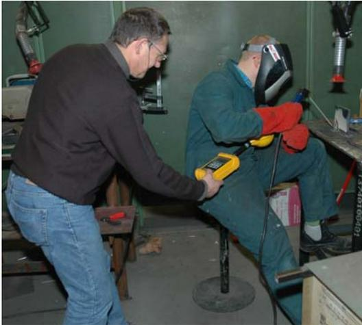
*B-field measurement on the welder's body*
