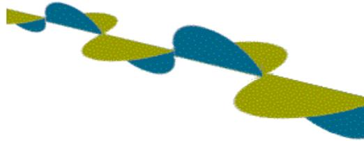
It is characterised by wave length, frequency and quantum energy. The lower the frequency, the lower the quantum energy, the longer the wave length and the longer the penetration depth.
