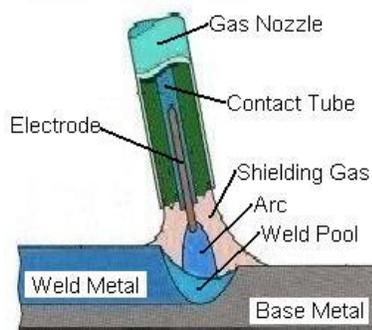
Gas Tungsten Arc Welding (GTAW) is frequently referred to as TIG welding. TIG welding is a commonly used high quality welding process. TIG welding has become a popular choice of welding processes when high quality, precision welding is required.
