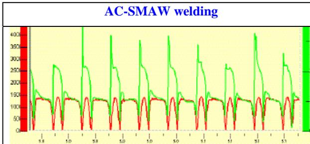
Figure 13: Voltage (green) and current (red) waveform
