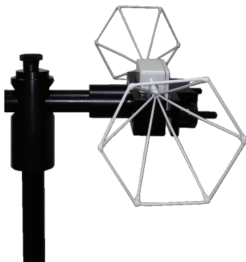
MPB biconical antenna: vertical and horizontal polarization
