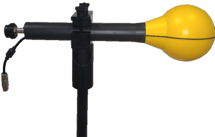
Narda SRM antenna: vertical and horizontal polarization
