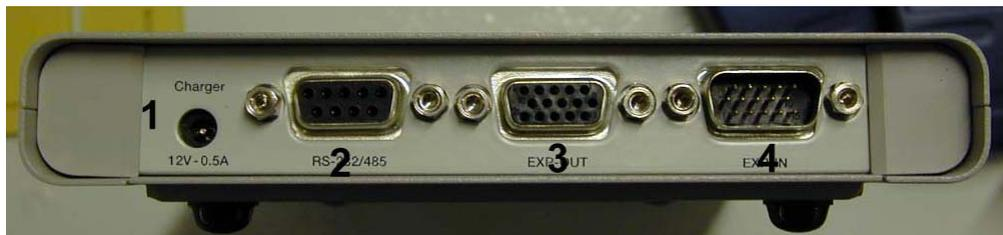
**Fig. 11-12 SB-04 Pannello posteriore**
