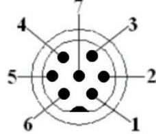
Fig. 3-7 "Remote Control" connector (Front view)
