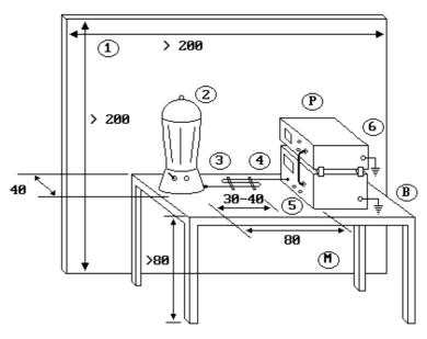
Fig. 5-1 Typical test set-up
