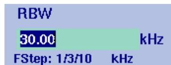
The input field allows you to enter a number or a text, depending on the selected function. The meaning of the input value is expressed by the header line. Some input fields have an additional explanation of the step size beneath. The step size applies when the value is changed using the up/down cursor keys instead of the numeric keys.
