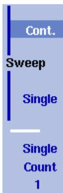
The 9102 can run measurements continuously or a defined number of times. Limiting the number of measurements can be useful for statistical analyses.
