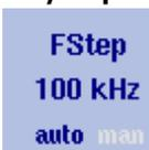
The center, start and stop frequencies can be set either by entering a new value with the numeric keys, or by using the arrow keys (**UP**, **DOWN**) to increase or decrease the current setting. The step size for an arrow keypress can either be selected automatically by the 9102, or manually adjusted.
