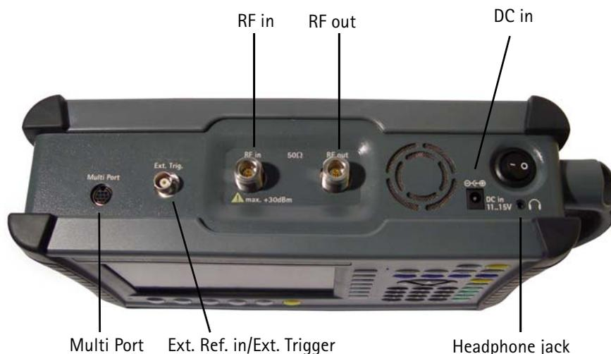
Figure 1 9102 connectors on the top of the instrument
