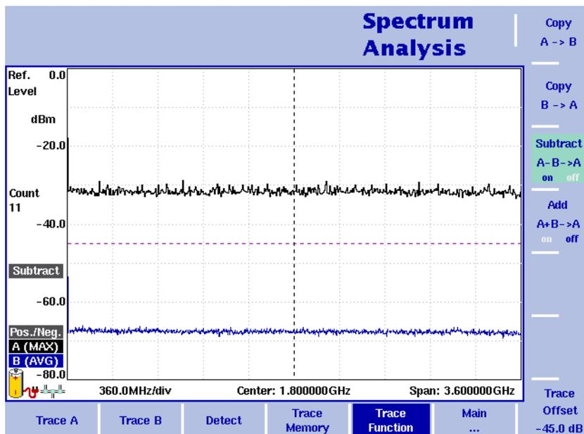
Figure 19 Subtract A - B → A on
