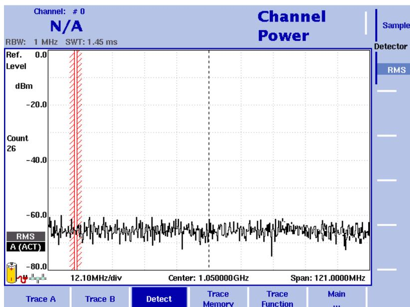
Figure 26 Detect menu with activated 9132 RMS Detector Option
