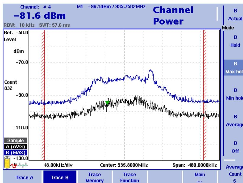
Figure 24 Example of a channel power measurement
