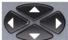
In an input field, the up and down cursor keys are used to increase or decrease the current value. The left and right cursor keys move the cursor position by one digit.
