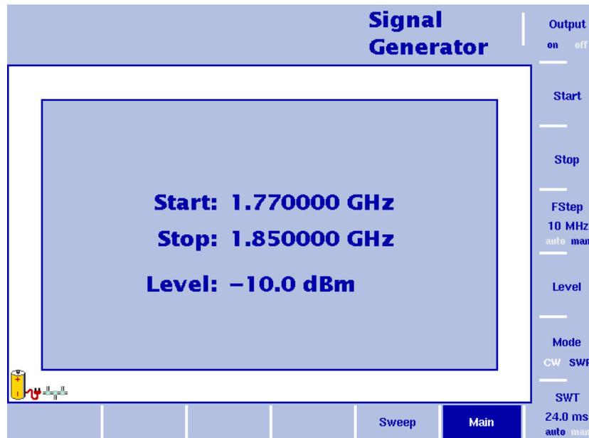
Figure 30 Signal Generator main menu in SWP mode
