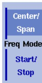
The Transmission main menu shows two softkeys for the definition of the frequency range on the display. Different methods exist to define the range as depicted above; you can configure these softkeys to one of the two allowable combinations as follows:
