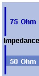
Most RF applications are using an impedance of 50  $\Omega$ ; other applications such as cable TV apply 75  $\Omega$ . The 9102 is designed with an input impedance of 50  $\Omega$ ; it can, however, be used for testing a device with an impedance of 75  $\Omega$  by using the software impedance switch. The measurement results from the 50  $\Omega$  input are recalculated to fit the different impedance.
