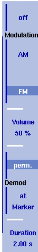
The 9102 has the ability to demodulate an AM (amplitude modulation) or FM (frequency modulation) signal and to output the signal at the built-in loud-speaker. The signal should have a signal strength of at least  $-50$  dBm; the demodulation bandwidth is about 10 kHz.
