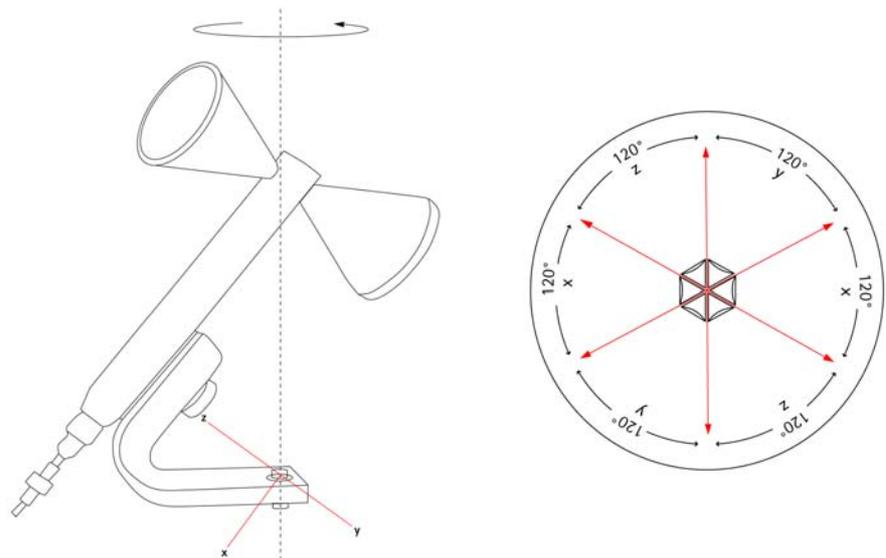
The 9102 supports consecutive measurements in three axes and automatically calculates the resulting field strength.
