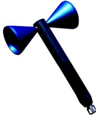
Biconical antennas are characterised by their dipole-like structure. The two reception lobes are highly symmetrical and provide the biconical antenna with two main reception directions with an opening angle of  $120^\circ$  each.
