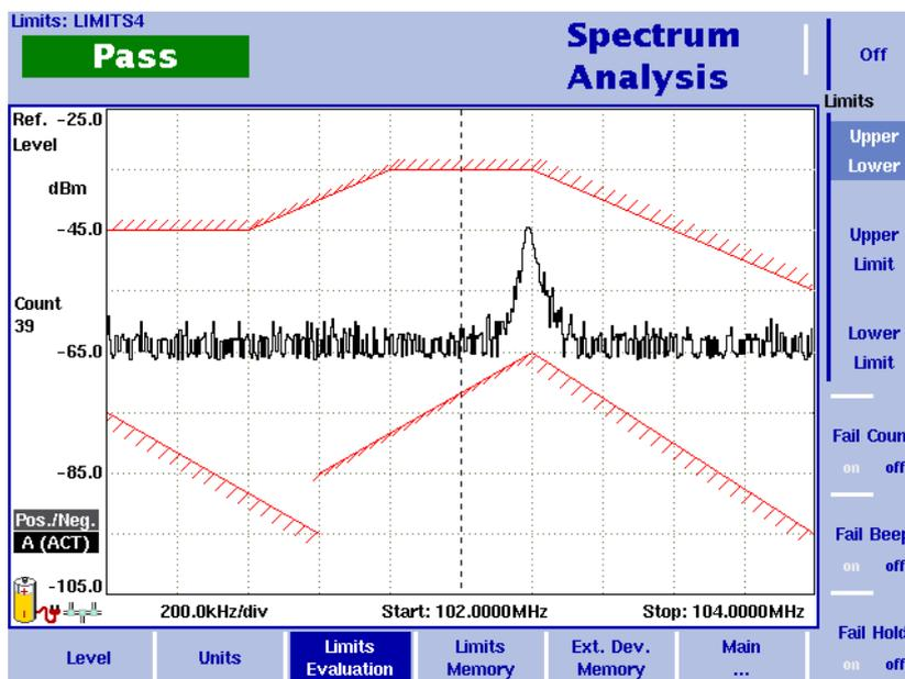
Figure 7 Example of limit lines in spectrum analysis
