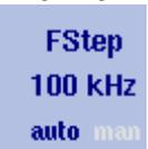
The center, start and stop frequencies can be set by either entering a new value with the numeric keys, or by using the arrow keys (**UP**, **DOWN**) to increase or decrease the current setting. The step size for an arrow keypress can be either automatically selected by the 9102, or manually adjusted.
