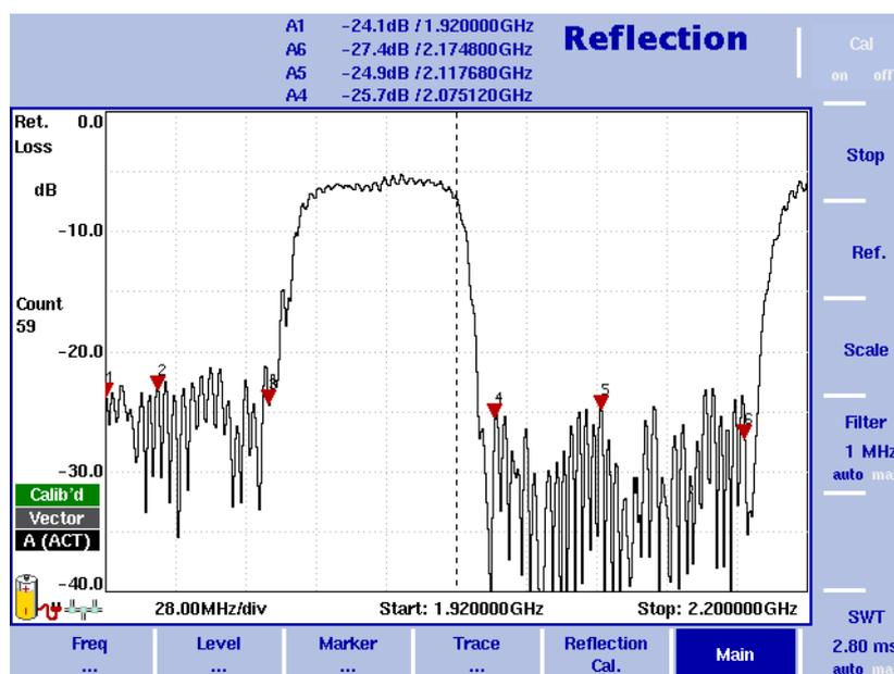
Figure 42 Example of a return loss measurement
