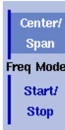
The Reflection main menu shows two softkeys for the definition of the frequency range on the display. Different methods exist to define the range as depicted above; you can configure these softkeys to one of the two allowable combinations as follows:
