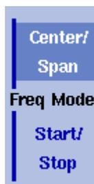
The Reflection main menu shows two softkeys for the definition of the frequency range on the display. Different methods exist to define the range as depicted above; you can configure these softkeys to one of the two allowable combinations as follows:
