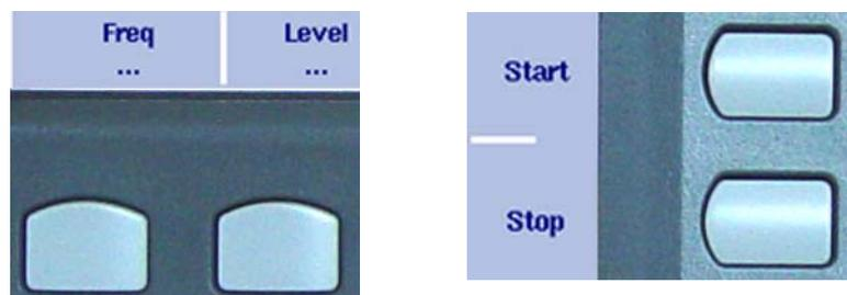
The softkey descriptions indicate the assignment of a function to a softkey. They are aligned to the lower side with the horizontal softkeys and to the right-hand side with the vertical softkeys. See ["Softkeys" on page 23](#) for more information.
