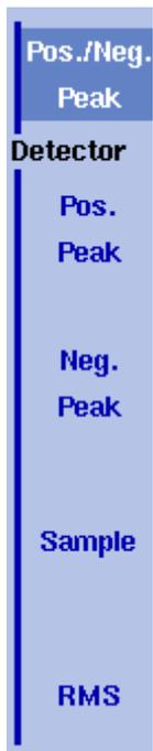
For each new measurement, the 9102 selects one or two values from a number of measurements for each frequency value. The method is user-definable; the following methods are available (see also [Figure 20](#)):
