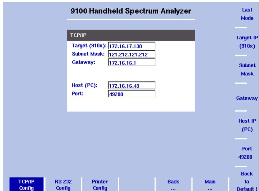
Figure 13 TCP/IP Configuration
