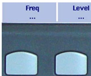
The horizontal softkeys provide access to the various menus. The name of the active menu is highlighted; the functions of a menu are offered on the vertical softkeys. Submenus are indicated with three dots ("..."); the menu softkey without the dots leads you one level up in the menu hierarchy.
