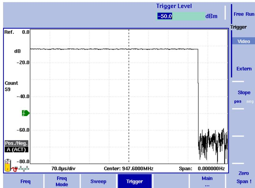
Figure 35 Triggered measurement (in the time domain)
