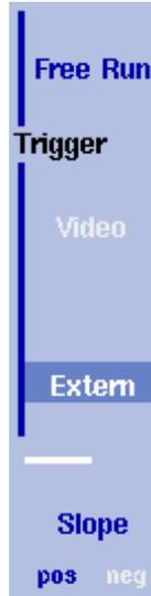
The 9102 can either start signal analysis at a random point in time, or start the measurement when a given signal threshold is passed. Starting measurements depending on the actual signal level is only supported in zero span mode.
