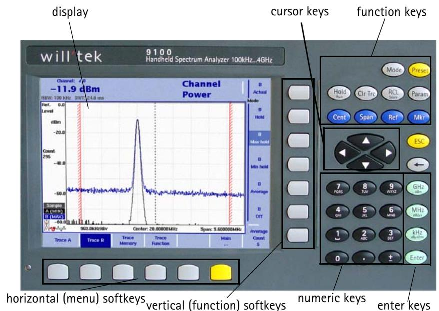
Figure 3 Front panel elements
