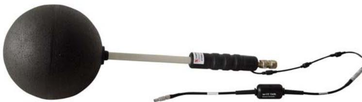
The most comfortable and fastest solution for performing EMF immission measurements comprises using an isotropic antenna. In an isotropic antenna three antennas or dipole elements, one for each direction (x, y and z), are arranged orthonogally and combined by interconnection as shown in the following graphic.
