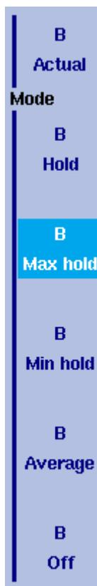
You can define two different trace views, e.g. one with the actual values and one with the maximum values. While the first view (Trace A) is always active, the second can be switched off. The functions of turning Trace B on or off and selecting the trace mode are combined as follows:
