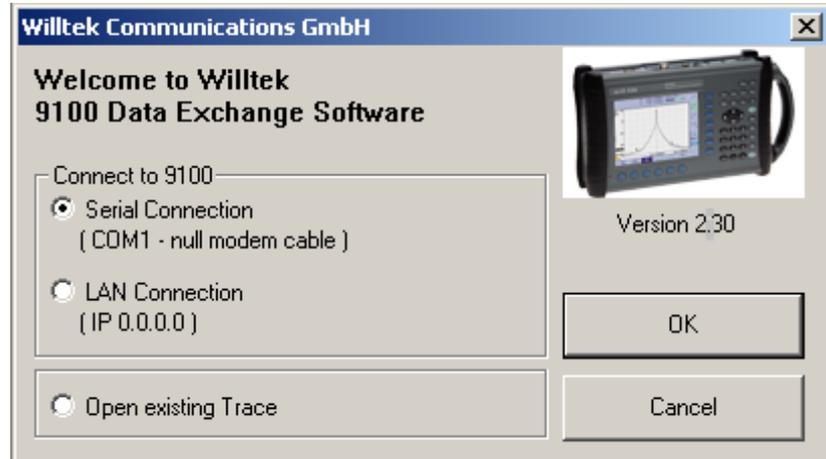
To connect to the 9102 via serial connection (RS-232 interface on a COM port of the PC), select **Serial Connection**.
