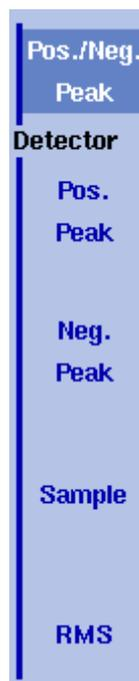
For each new measurement, the 9102 selects one or two values from a number of measurements for each frequency value. The method is user-definable; the following methods are available (see also [Figure 37](#)):
