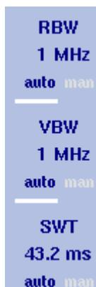
The resolution bandwidth (RBW) is the 3 dB bandwidth of the IF filter for selecting the signal to be measured. The resolution bandwidth describes the ability of the spectrum analyzer to discriminate between adjacent signals of similar amplitude. Only signals spaced at a frequency of more than the RBW can be discriminated from one another.
