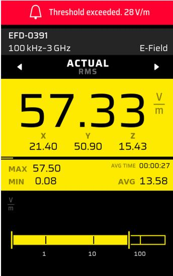
Fig. 18: Display of alarm function
