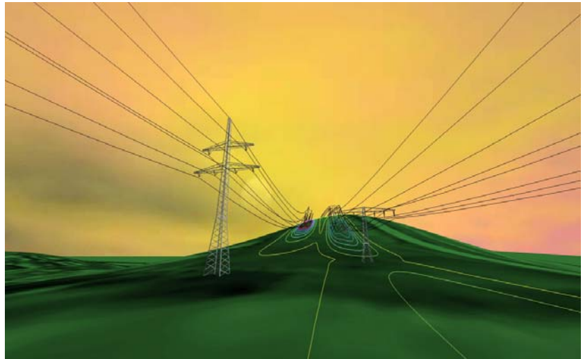
Fig.: magnetic field of terminal stations
