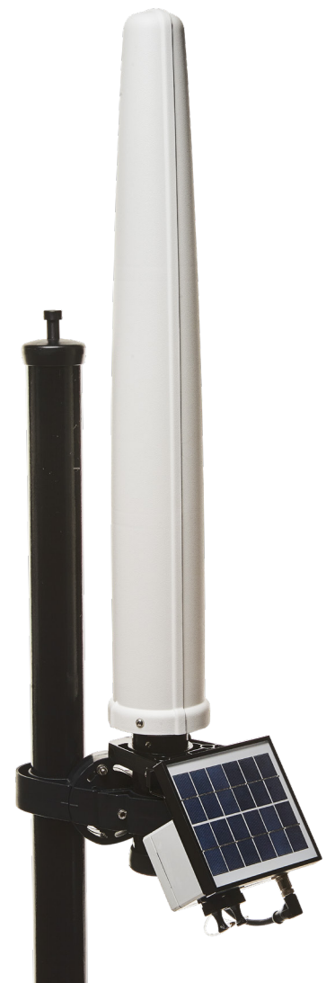
Area Monitor AMB-8059/03 with Solar Panel
