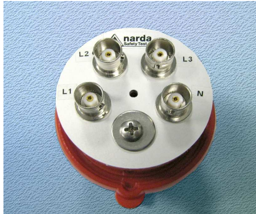
A-D-17 PMM L3-32 model adapter (32 A sockets)
