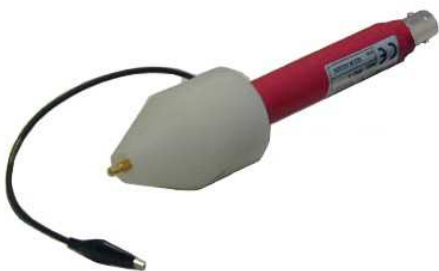
Fig. A-D-13 SHC-1/1000: 35 dB CISPR Voltage probe
